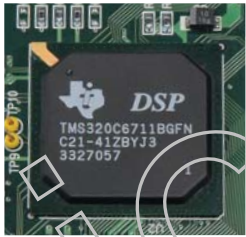
● 32-Bit High-Speed Floating-Point DSP
