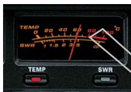
●Final Amplifier Temperature Display (MP/Contest Versions)
